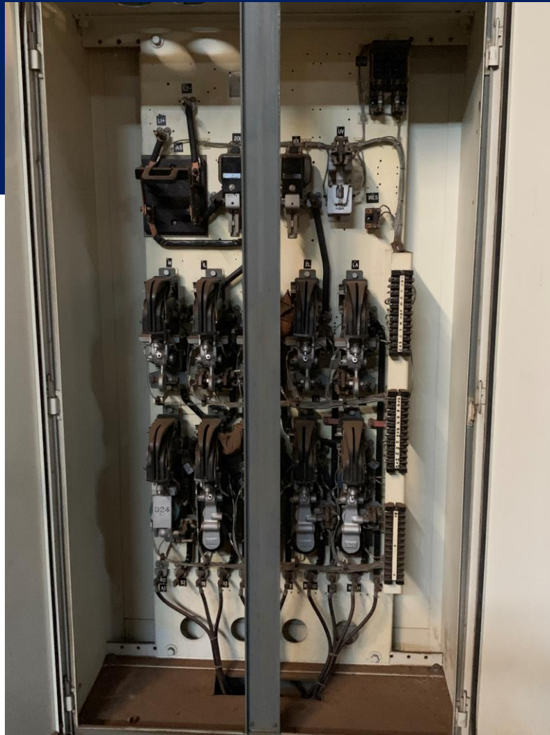
(2) Nema Size 4, 33 HP, 230 Volt DC, Cutler Hammer Hoist Control Panel, Front Wired, 5-Speed, 900 Series Contactors, Dynamic Lowering, Mounted in Enclosure, complete with resistors mounted in fabricated steel racks
